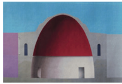
Figure 6 - Section diagram of the elliptical dome structure @ Nisa
